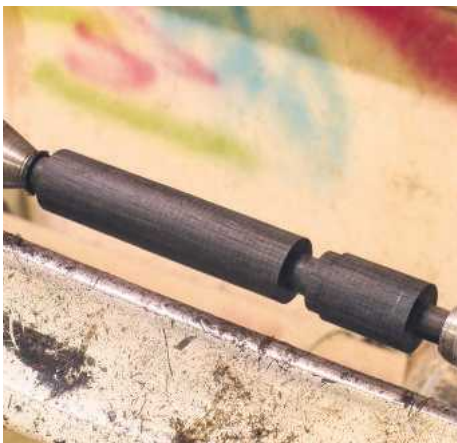
▲ Pic.25 All the important sizing cuts are now done. The small fillet above the top spigot is the right diameter for the flat on the top. Take care that the piece doesn't become too weak
